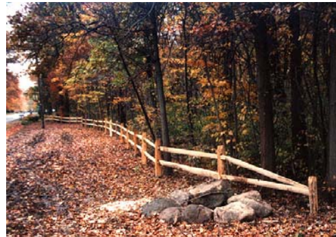
Two rail split rail fencing, 3 feet high
